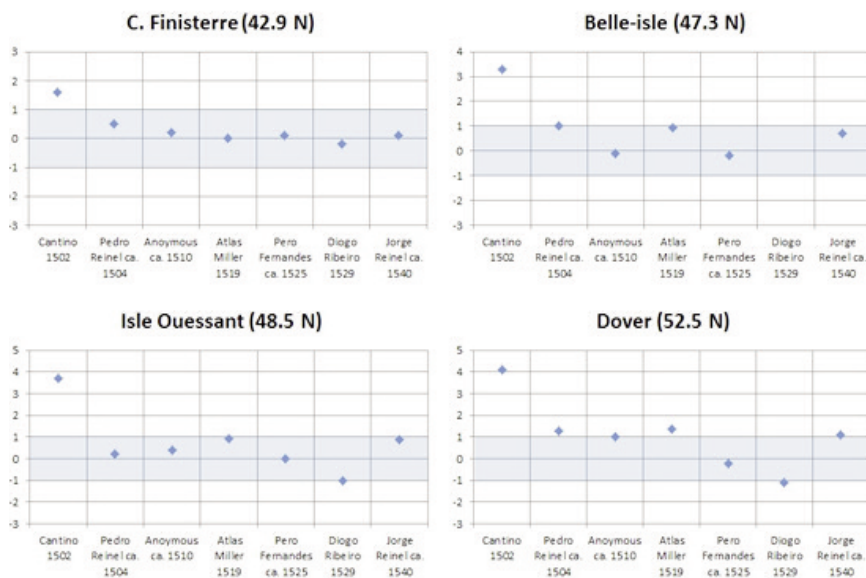
Figure 6 : Latitude errors in a sample of nautical charts of the first half of the sixteenth century, for four places in northern Europe. With very few exceptions the errors become less than one degree from about 1504
